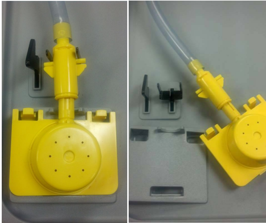
Figure 4: Nozzle Assembly Removed
