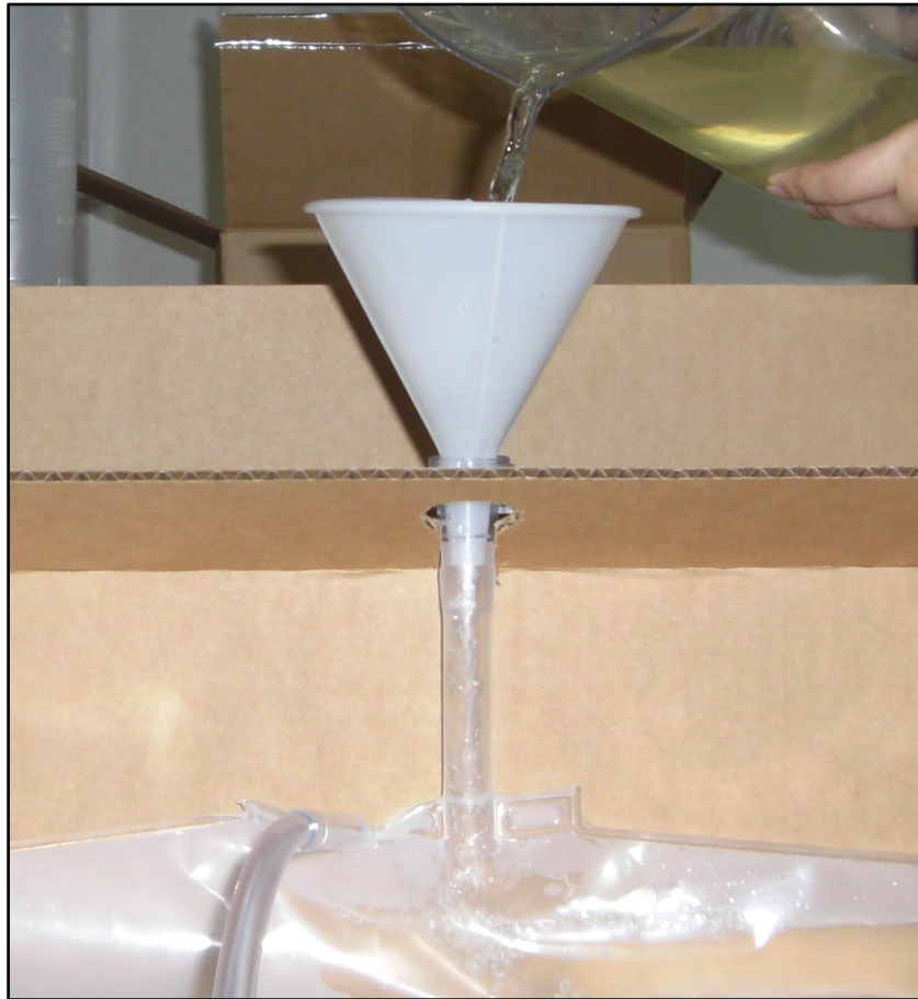
Figure 5: Funnel installed for filling.
