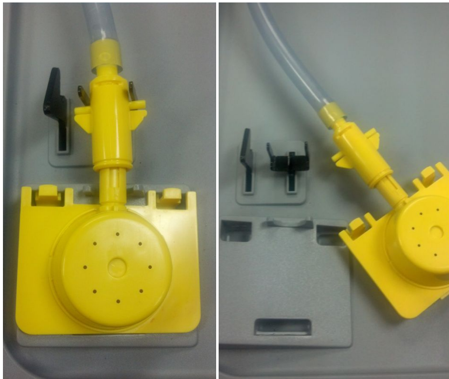
Figure 4: Nozzle Assembly Removed
